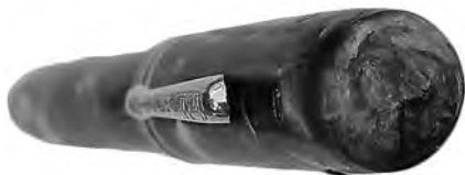
Conklin cap, showing advanced crazing.
